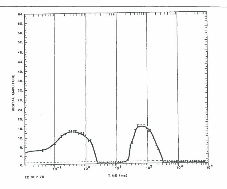
FIG. 3. BHANGMETER OPTICAL TRACE NO. 2
