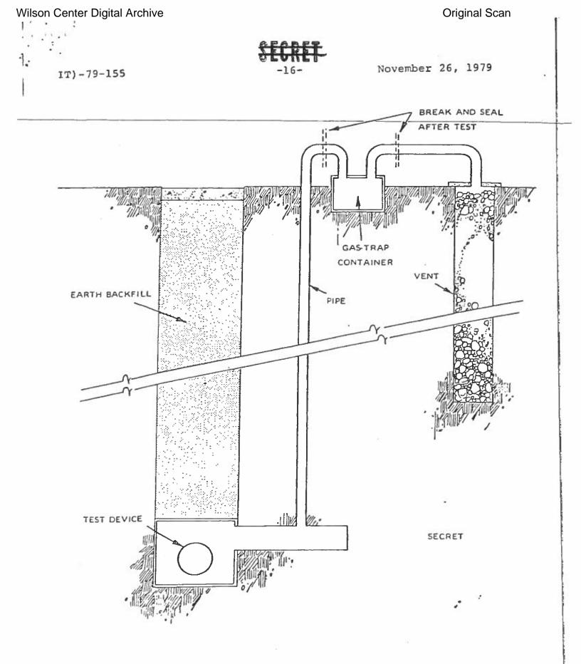
FIG. 7. PROFILE OF TEST GEOMETRY FOR ABOVE GROUND SAMPLING
