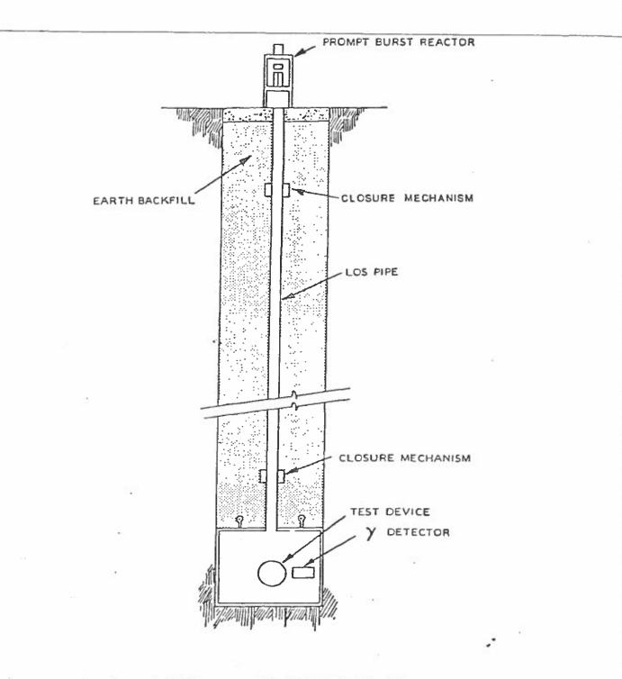
FIG. 5. PROFILE OF TEST GEOMETRY FOR NEAR-ZERO YIELD NUCLEAR TESTS
